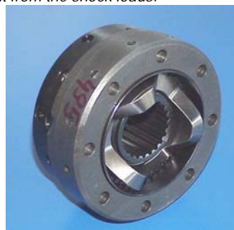
Photo #7 – The overload clutch shown here is now standard equipment on all new 912 series engines. Older engines can be retrofitted for protection from propstrikes and smoother operation.
