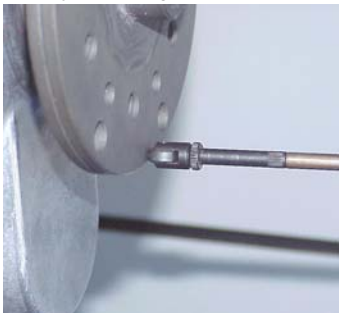
Photo #1 – Check the prop Flange for run out. Maximum of .003" is allowable.
