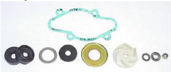
Figure #6 – Several parts after seal pair are now considered optional. The freeze plug and associated parts help prevent seal walk.
