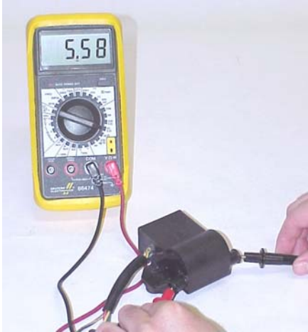
Figure #5 – Here we test the output leads of our E-Box. The range is from 5100 to 6300 ohms. With our meter set to the 20K ohms range we find 5580 ohms. The circuit test good. You can do this with the plug wires attached and the plug caps removed.
