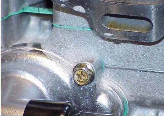
Photo #5 – Pressurizing the system to +5 psi and spraying the block with a solution of 50% water and 50% liquid dishwashing soap will pinpoint any leak. Here we have loosened a water pump housing bolt during the cooling system test to show the bubbles created by a leak.
